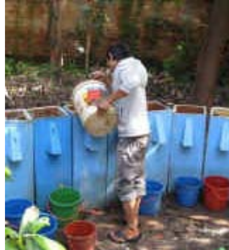
Photograph 1. Filling the filters at 40 L/day
